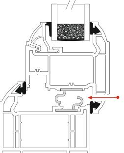
**STAY GUARD ELITE SG026** on outer frame and sash for all types of stays to include Egress/Easy Clean
